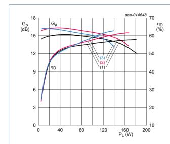
$V_{DS}$  = 28 V;  $I_{Dq}$  = 250 mA (main device);  $V_{GS(amp)peak}$  = 0.7 V;  $t_p$  = 100  $\mu s;$   $\delta$  = 10 %.
