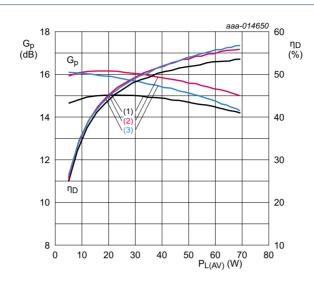
$V_{DS}$  = 28 V;  $I_{Dq}$  = 250 mA (main device);  $V_{GS(amp)peak}$  = 0.7 V.
