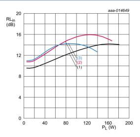
$V_{DS}$  = 28 V;  $I_{Dq}$  = 250 mA (main device);  $V_{GS(amp)peak}$  = 0.7 V;  $t_p$  = 100  $\mu s;$   $\delta$  = 10 %.
