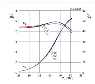
$V_{DS}$  = 28 V;  $I_{Dq}$  = 800 mA;  $V_{GS(amp)peak}$  = 1.0 V.
