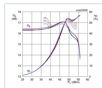
$V_{DS}$  = 28 V;  $I_{Dq}$  = 800 mA;  $V_{GS(amp)peak}$  = 1.0 V.
