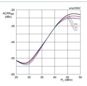
$V_{DS}$  = 28 V;  $I_{Dq}$  = 800 mA;  $V_{GS(amp)peak}$  = 1.0 V.
