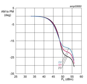
$V_{DS}$  = 28 V;  $I_{Dq}$  = 800 mA;  $V_{GS(amp)peak}$  = 1.0 V.
