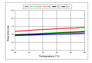
Figure 12. 20%-80% Rise Time vs Temperature
