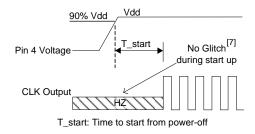
Figure 4. Startup Timing (OE/ST Mode)
