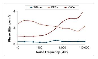
Figure 4. Power Supply Noise Rejection<sup>[4]</sup>
