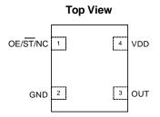
Figure 1. Pin Assignments
