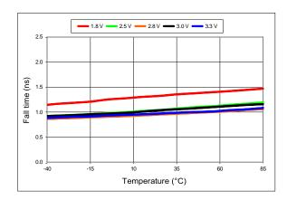
Figure 13. 20%-80% Fall Time vs Temperature
