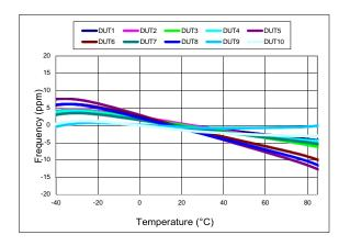
Figure 9. Frequency vs Temperature
