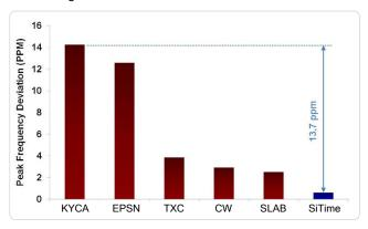
Figure 6. Shock Robustness<sup>[6]</sup>
