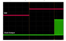
Figure 18. Startup Waveform vs. Vdd
