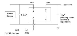
Figure 2. Test Circuit
