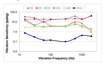
Figure 5. Vibration Robustness<sup>[5]</sup>
