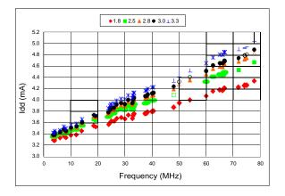
Figure 8. Idd vs Frequency
