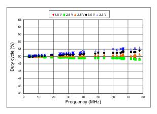
Figure 11. Duty Cycle vs Frequency
