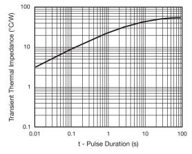
Fig. 6 - Typical Transient Thermal Impedance
