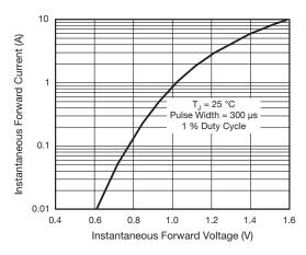
Fig. 3 - Typical Instantaneous Forward Characteristics
