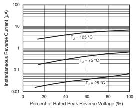
Fig. 4 - Typical Reverse Characteristics
