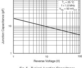
Fig. 5 - Typical Junction Capacitance
