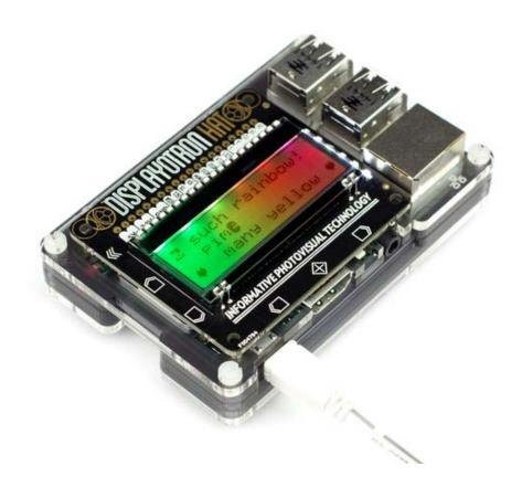
Great for including a colourful character display and button inputs on your Raspberry Pi based projects! Includes a 16x3 character LCD display, 6-zone RGB LED backlight, bar graph, and six capacitive touch buttons all in one slim package.
